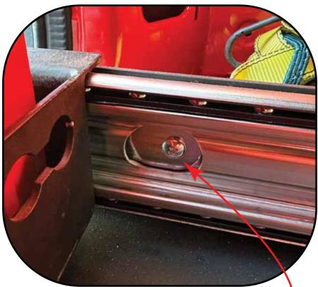
ACCESS HOLE FOR SLIDE MOUNT SCREWS
