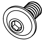
1/4-20 X 0.5 FLANGED BUTT HEAD HEX DRIVE SCREW
