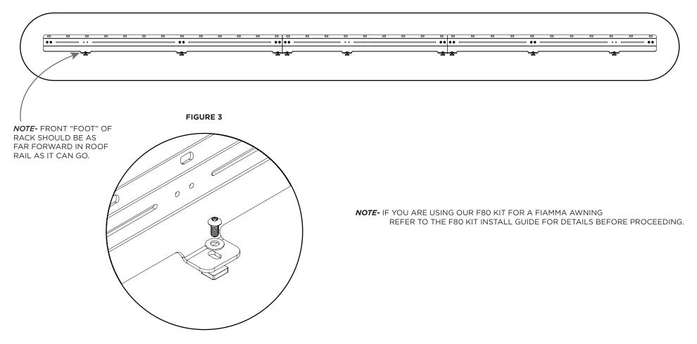
**4.** PLACE YOUR CROSSBARS IN DESIRED LOCATION, LOOSELY BOLTING THE 1/4-20 FLANGE HEAD SCREWS IN PLACE.
